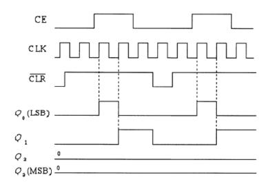
10. The waveforms in Figure 8-75 are applied to a 74HC163 binary counter. Determine the Q outputs and the RCO. The inputs are  $D_0 = 1$ ,  $D_1 = 1$ ,  $D_2 = 0$ , and  $D_3 = 1$ .
